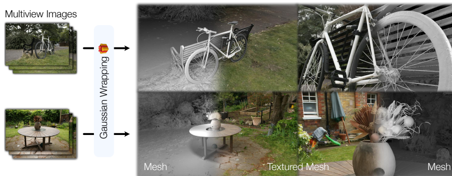
Fig. 1: High-fidelity surface reconstruction from 3D Gaussian Splatting. Our method, Gaussian Wrapping, reconstructs watertight and textured surface meshes of full 3D scenes given multiview RGB images, by interpreting 3D Gaussians as stochastic oriented surface elements. This figure illustrates the resulting surface meshes, with and without the RGB texture. Our meshes represent the full scene—including background geometry and extremely thin structures such as bicycle spokes where existing methods fail—with a significantly more compact representation than concurrent works [10, 57].
